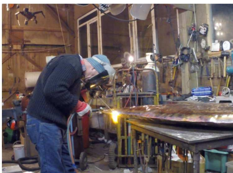
The brazing process using bronze wire and oxyacetylene
