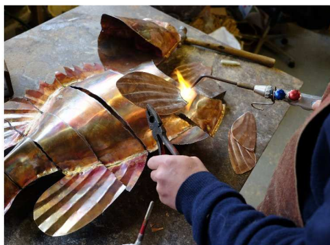
The fish is cut into eight sections fins added and then balanced
